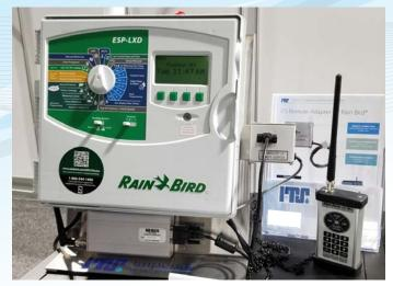
Allows direct controller communication between the Rain Bird controller and the Rain Master Pro-Max Remote System.
